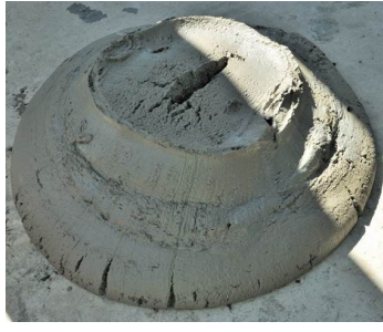
Paste Thickeners Underflows. On the left, a mud with a yield stress of 110 Pascals. On the right, a 450 Pascal yield stress
